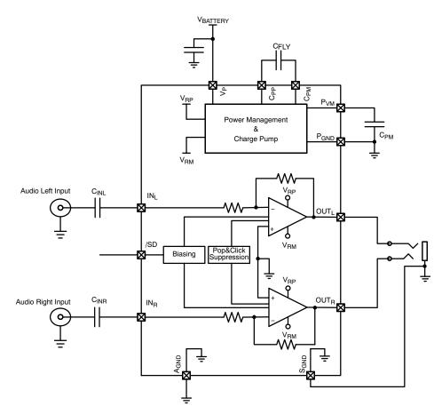
Figure 12. Typical Application Circuit
