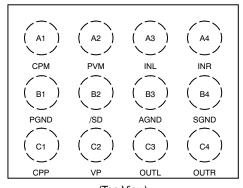
(Top View) 12-Pin 1.2 x 1.6 mm CSP
